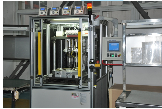
热熔焊接 Hot Melt Welding
